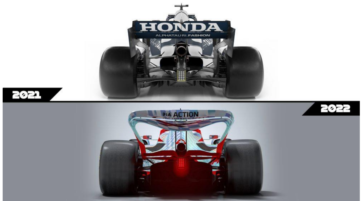
Figure 12. A comparison of the 2021 and 2022 rear wing designs. (Reynolds, 2021)
