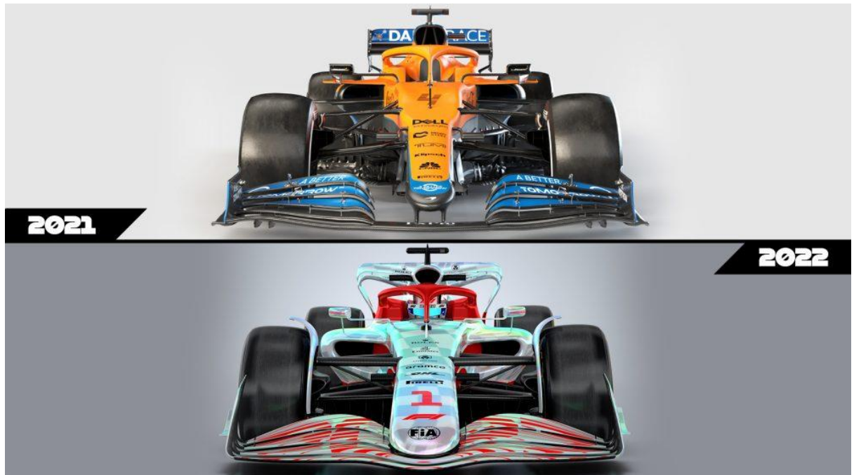
Figure 11. A comparison between the 2021 and 2022 front wing designs. (Hughes & Piola, 2022)
